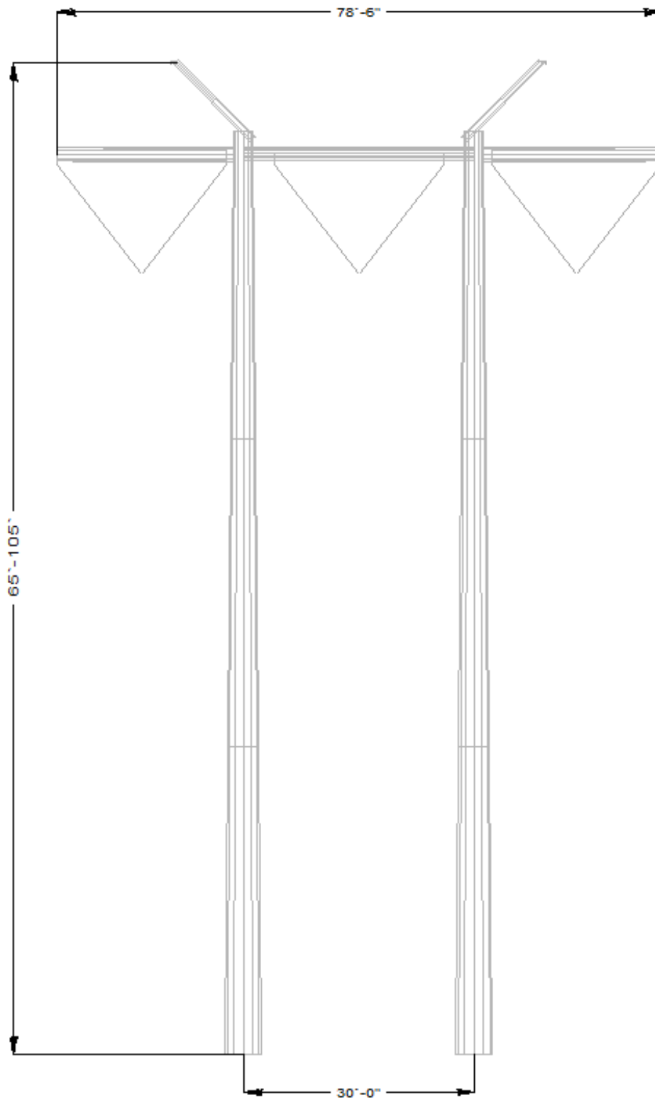
Figure B-17. Proposed/Alternative 500-kV Single-Circuit Tubular Steel Pole H-Frame Structure
