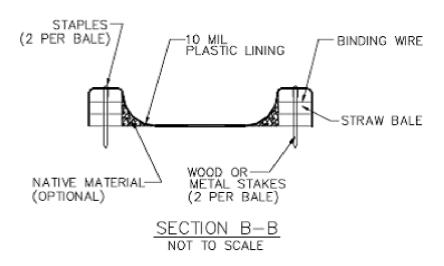
Figure G-1. Example of Typical Spill Containment Area
