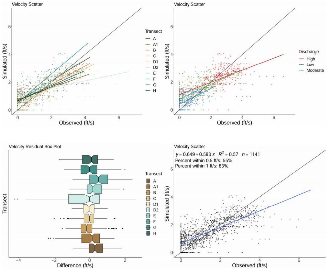
Figure D-2. Linear regression of simulated compared to observed velocity at each transect (top left), combined by flow (top right), velocity residual error at each transect (bottom left), and for all comparison data combined (bottom right).
