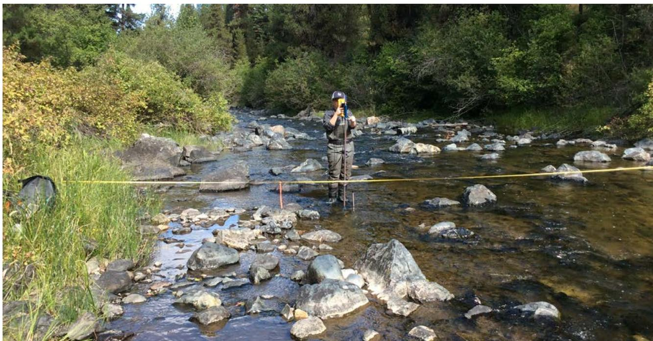
**Figure 11 Photograph of CFS staff using the FlowTracker2 to record depth, velocity, and discharge at transect F during Low calibration discharge field collection.**
