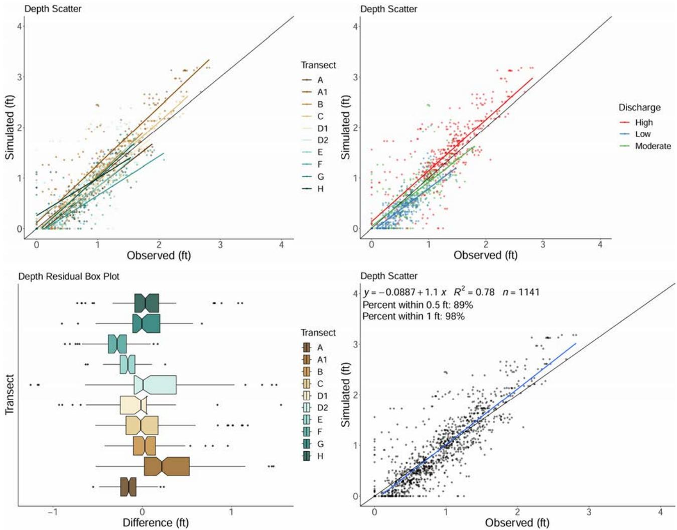
Figure D-1. Linear regression of simulated compared to observed depth at each transect (top left), combined by flow (top right), depth residual error at each transect (bottom left), and for all comparison data combined (bottom right).
