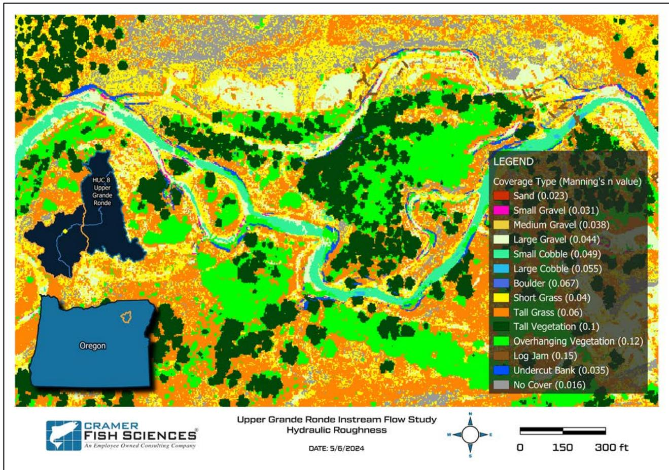
**Figure 17. Example of the hydraulic roughness spatial coverage.**
