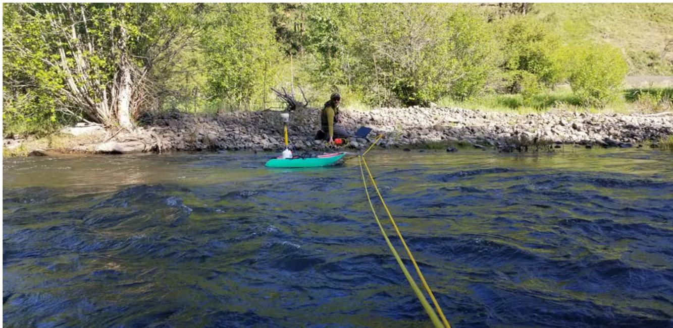
**Figure 10 Photograph of CFS staff using the SonTek M9 to record depth, velocity, and discharge at Transect D during High calibration discharge field collection.**
