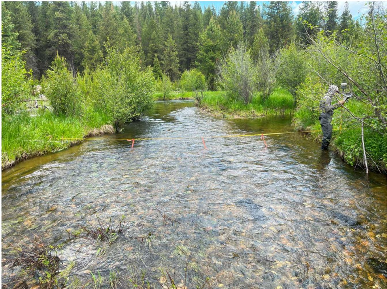
**Figure 9 Photograph of CFS staff taken at Transect G during the Moderate discharge field data collection, showing a flagged tape strung across the transect location.**
