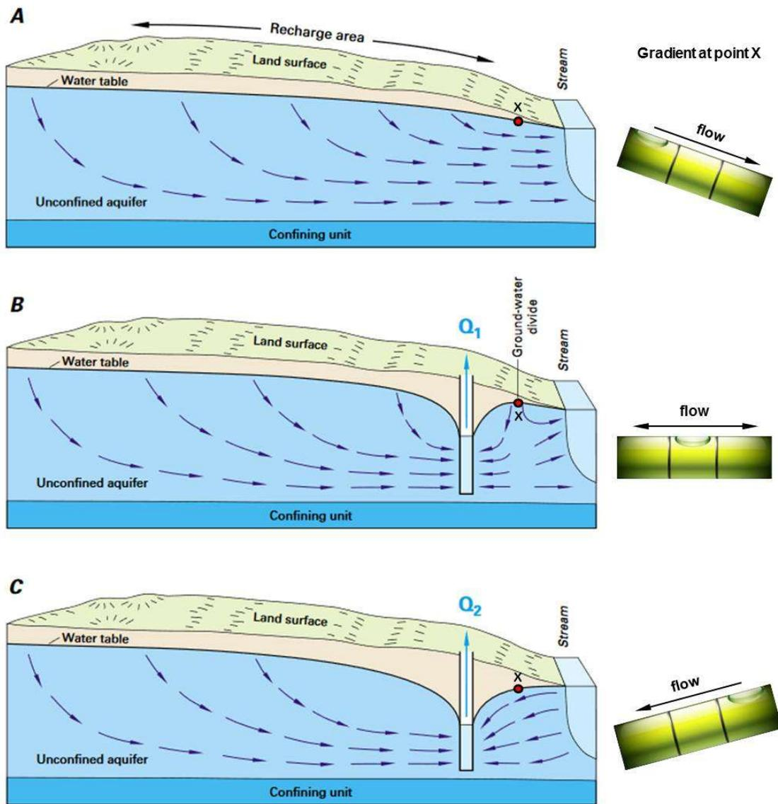
Figure 6. Adapted from Alley, 1999. Diagram showing the development of groundwater capture at two different pumping rates ( $Q_1 < Q_2$ ) and the impact of pumping rates on hydraulic gradient and ultimately, flow path direction.
