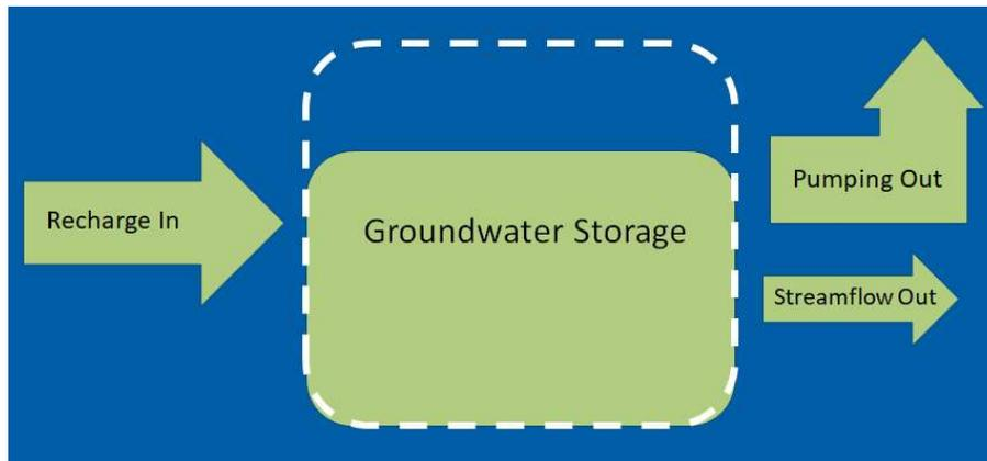
*Figure 4. A new equilibrium is established when groundwater discharge decreases, in this example because discharge to rivers and streams has decreased significantly and discharge to pumping has decreased minimally.*
