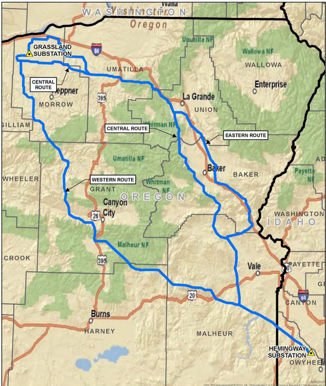
FIGURE 3.4-6 WESTERN, CENTRAL & EASTERN ALTERNATIVES IDAHO POWER COMPANY BOARDMAN TO HEMINGWAY 500KV TRANSMISSION LINE PROJECT AUGUST 2010 Substation Alternative State Boundary County Boundary LOCATION MAP
