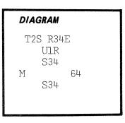
from which: A pine, 24 ins. diam., bears N49°30'W., 252 lks, dist. marked U1R64M BT. A pine, 6 ins. diam. bears N21°45'E., 133 lks. dist. marked U1R64M BT."
