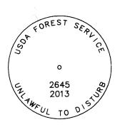
SET A 5/8" X 30" REBAR WITH A 3  $\frac{1}{4}$ " ALUMINUM CAP MARKED AS SHOWN (TYPICAL)
