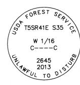
SET A 3" X 30" PIPE WITH A 3  $\frac{1}{4}$ " ALUMINUM CAP MARKED AS SHOWN.
