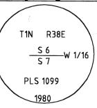
Set: by single proportionate measurement, a 2" x 30" galvanized iron pipe, 28" in the ground, with brass cap, from which:
