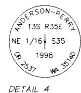
SET A 2 1/2 INCH ALUMINUM CAP ON A 5/8 INCH IRON ROD, 2 INCHES ABOVE GROUND AND SURROUNDED BY A 2 FOOT DIAMETER MOUND OF STONE WITH THE CAP MARKED AS SHOWN.
