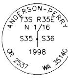
SET A 2 1/2 INCH ALUMINUM CAP ON A 5/8 INCH IRON ROD, 4 INCHES ABOVE GROUND AND SURROUNDED BY A 3 FOOT DIAMETER MOUND OF STONE WITH THE CAP MARKED AS SHOWN.
