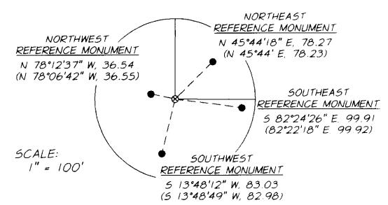
THE LOCATION OF THE SOUTHWEST CORNER OF SECTION 35 WAS ESTABLISHED AT THE MEAN COORDINATE POSITION OF FOUR DIS-TANCE/DISTANCE INTERSECTIONS USING RECORD MEASUREMENTS FROM REMONUMENTATION RECORD 003-1995R.
