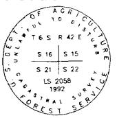
FROM WHICH G.L.O. ACCESSORIES: A DEAD AND DOWN PINE, 32" DIAM. [10"], BEARS S45"20"V [\$47'W], 50.11' [49.5'], SCRIBING NOT MSIBLE. A PINE STUMP, 24" [24"] DIAM. BEARS \$65'28'E [\$72'E], 134.92' [130.7'], BLAZE NOT VISIBLE A FIR STUMP, 24" [5"] DIAM, BEARS N28E [N28E]
