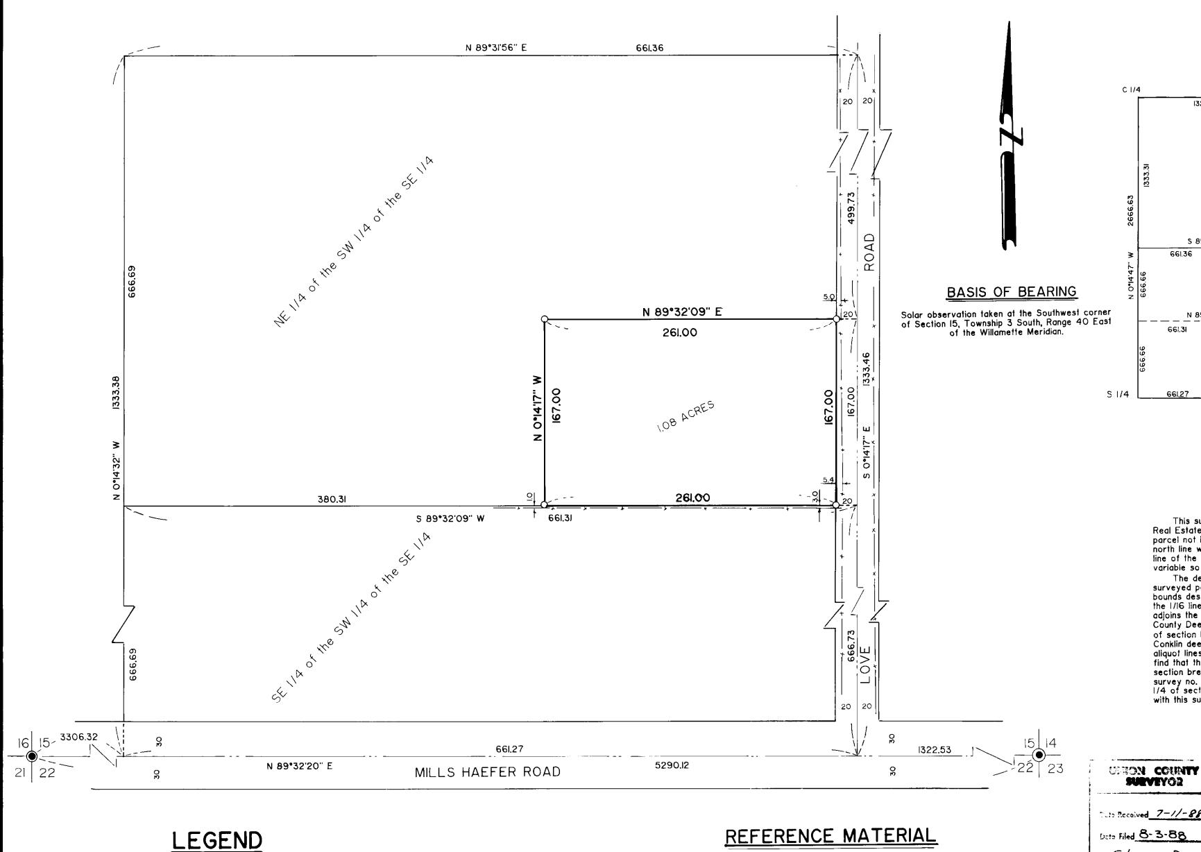
Set 5/8" × 30" iron pin with plastic cap marked BGA SURVEY MARKER. Found brass cap monument as per
