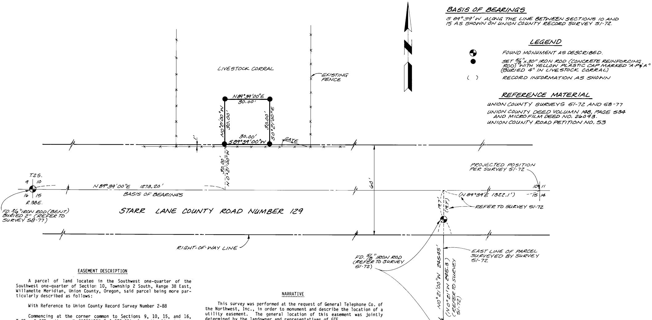
Commencing at the corner common to Sections 9, 10, 15, and 16, T.2S., R.38E., thence N 89°39'00" E 1,273.20' along the line between Sections 10 and 15 to a point, thence N 0°21'00" W 30.00 to a point on the Northerly right-of-way line of Starr Lane County Road Number 129 and the TRUE POINT OF BEGINNING OF this Easement Description;
