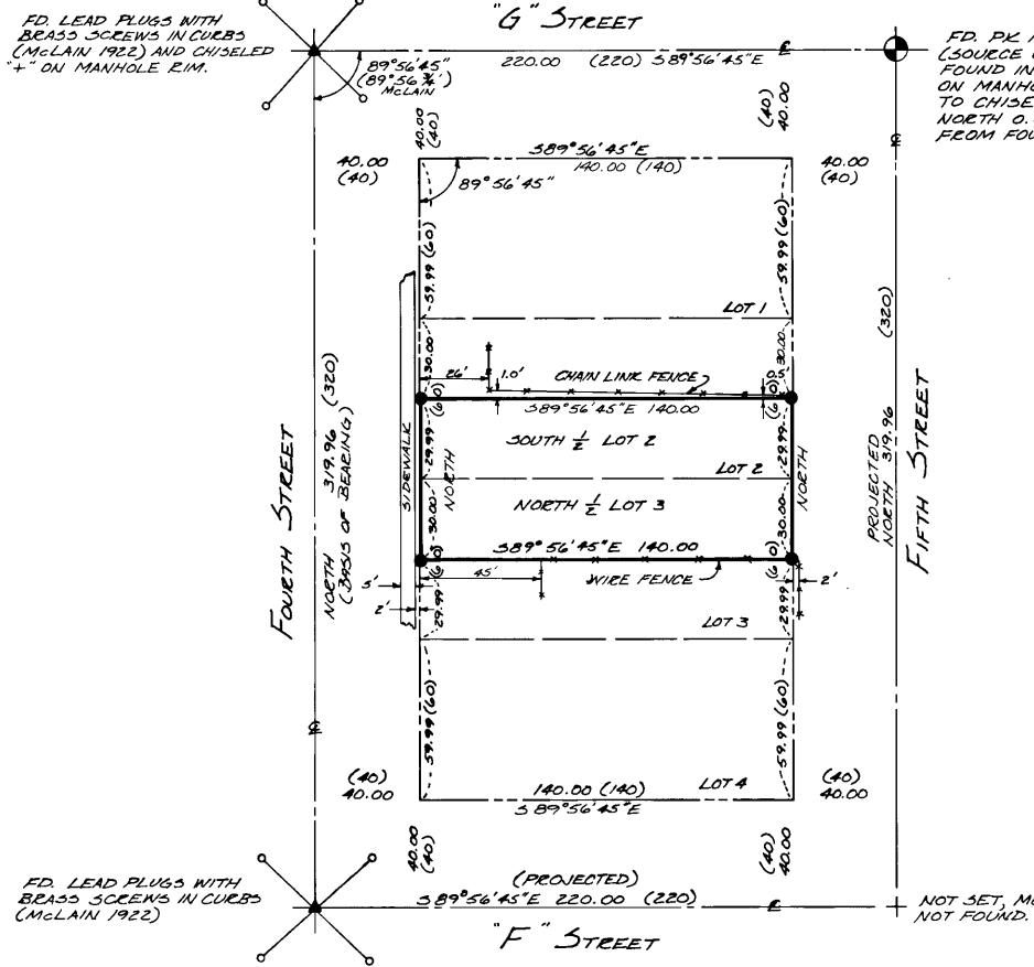
FD. PK NAIL IN ASPHALT (SOURCE UNKNOWN). ALSO FOUND INTERSECTION POINT ON MANHOLE LID (BY REFERENCE TO CHISELED "+" ON RIM) BEARS NORTH 0.05' AND EAST 2.63' FROM FOUND PK NAIL.
