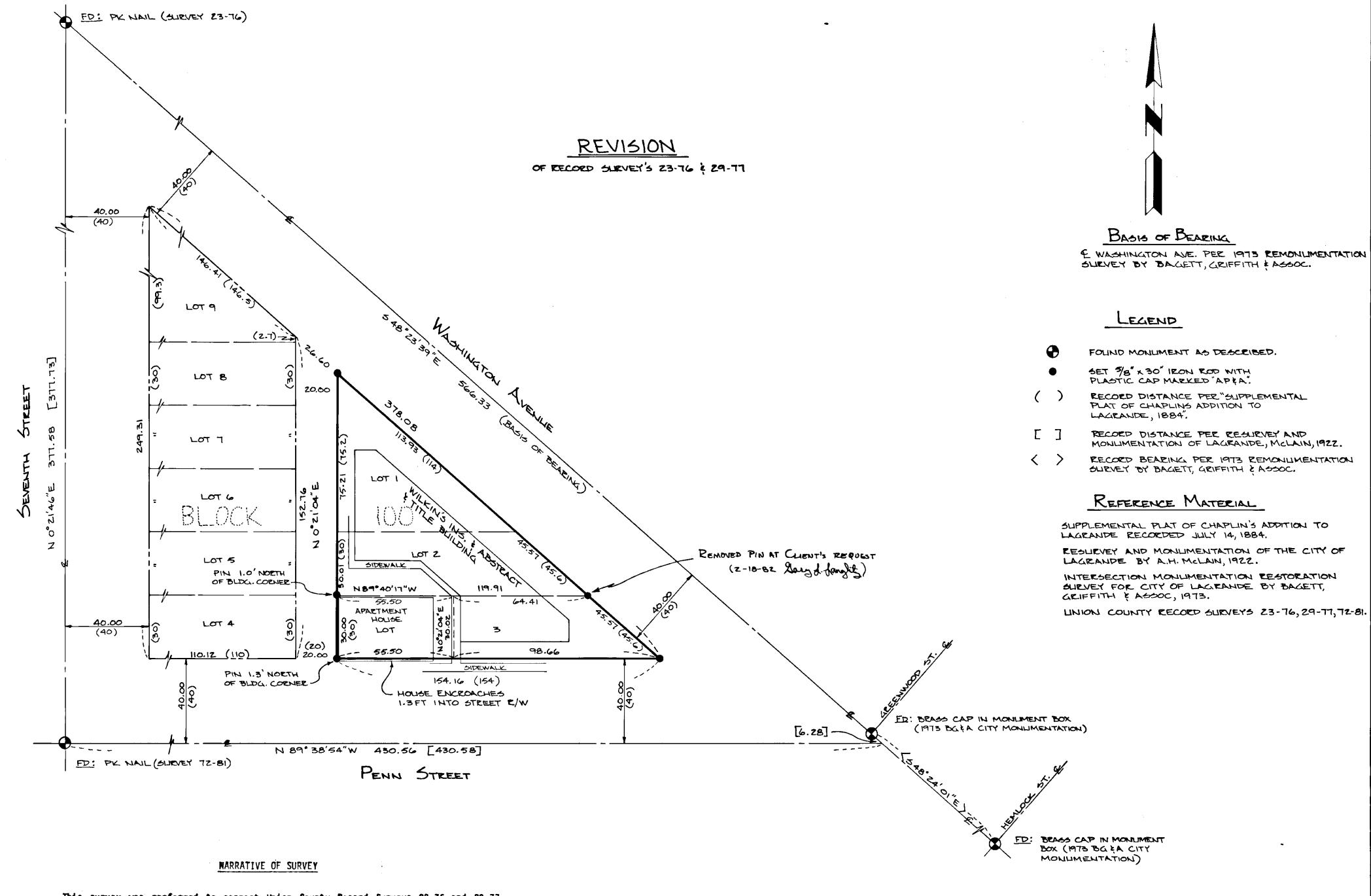
This survey was performed to correct Union County Record Surveys 23-76 and 29-77. These prior surveys incorrectly placed the centerline intersection of Penn Street and Washington Avenue at the monumented centerline intersection of Washington Avenue and Greenwood Street. A careful review of the field notes and plat of McLain's 1922 survey shows the centerline intersection of Penn Street to be SE of the Greenwood Street intersection along the centerline of Washington Avenue as shown on this map.
