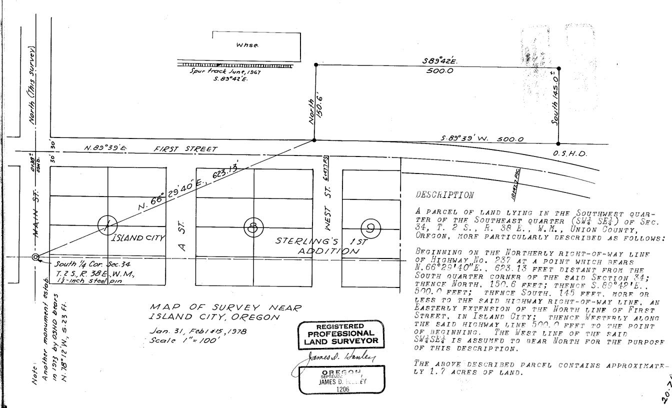
The purpose of this survey was to establish the Southeast corner of the parcel along the North line of the old O.S.H.D. right of way, which was an extension of the North line of First Street.
