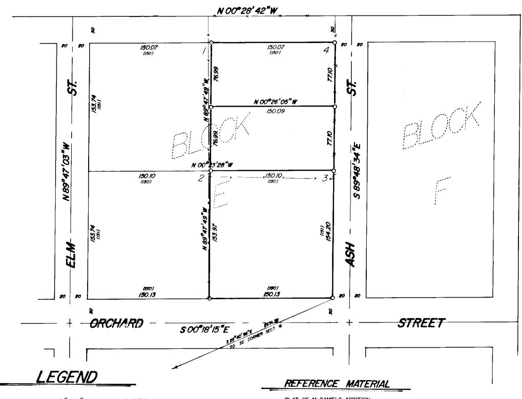
SET 5/8"x 30" IRON PIN WITH PLASTIC CAP MARKED B.G.A SURVEY MARKER
