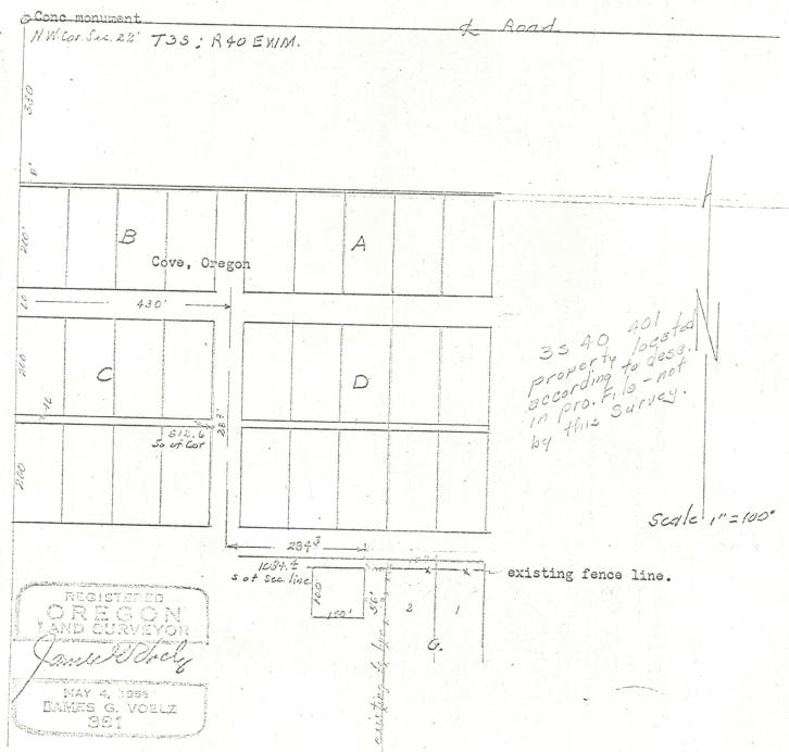
A tract of land lying in the NW+NW+ of Section 22, T3S, R40EWM and described as follows; Commencing at a point 1084.4 ft. south and 714.3 ft. east of the Northwest corner of said section 22, said point being on the south line of water street extended, (said point formerly described as being 70 ft. west of the northwest corner of lot 2 Block G of The Town of The Cove) thence south and parallel to the west line of said lot 2 Block G 100 ft. Thence at right angles west 100 ft.;
