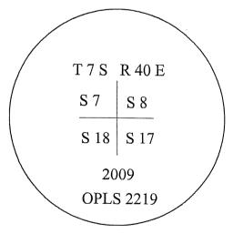
I used a steel tape and magnetic compass in the establishment of the new accessories. I used 18° East declination, the distances are to a center of the aluminum cap.
