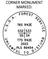
Painted a 6 inch red band around the bearing tree, and also painted blazes red. Attached USFS 54-3 and 54-9 signs to BT. Distance to bearing tree was measured with a steel tape to a 60d nail driven in the side-center at the root crown of the tree, with an attached 1½" aluminum washer stamped PLS 69454. Used RTK GPS to measure accessories. Bearings are geodetic, derived by GPS observation at the corner. Set an aluminum guard post North, 2.5 ft. with USFS 54-2 and 54-9 signs attached.
