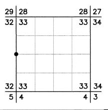
**ORIGINAL DESCRIPTION:** Set basalt rock 14x12x6 ins., 10 inches in ground for 1/4 Sec. corner, marked 1/4 on the West face, from which
