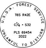
Used RTK GPS to measure accessories. Bearings are geodetic, derived by GPS observation at the corner.
