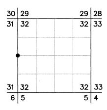
**ORIGINAL DESCRIPTION:** Set basalt rock 12x10x6 ins., 8 inches in ground for 1/4 Sec. corner, marked 1/4 on the West face raised mound of rock alongside. Pits impracticable.
