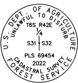
Deposit K-tag north and alongside the pipe. Also placed a plastic-encased magnet at base of pipe. Used RTK GPS to measure accessories. Bearings are geodetic, derived by GPS observation at the corner.
