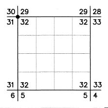
**ORIGINAL DESCRIPTION:** Set basalt rock 16x12x4 ins., 11 inches in ground for corner to Sec 29, 30, 31, 32 marked with 1 notch on the South and 5 notches on the East edges, raised mound of rock alongside, pits impracticable
