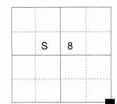
Section Corner Stone 5"x12"x18" located South 114.5' from Sta 32+73.
