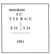
A larch, 14 ins. diam., bears N.21°E., 80 lks. dist. mkd. T5S R41E S34 SC BT. A fir, 20 ins. diam., bears N.61°W., 70 lks. dist. mkd. T5S R41E S33 SC BT.
