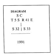
A root hole with burned wood within, bears N.50°E., 33 lks. dist. A rotten remains of a pine stump, upright in place, size indeterminate, bears N.30°W., 78 lks. dist. no marks.
