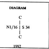
A stainless steel post, 28 ins. long, 2½ ins. diam., set 22 ins. in the ground, for a reference monument, bears S.54°15′W.,0.412 chs. dist., with brass cap mkd. RM CN 1/16 S34 27.2 FT TO COR 1992 and an arrow pointing to the corner. Set a steel fence post alongside the reference monument. A ponderosa pine, 25 ins. diam., bears N.17°W., 61 lks. dist. mkd. CN 1/16 S34 BT.
