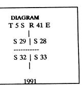
A lodgepole pine, 12 ins. diam., bears N.45½°E., 136 lks. dist. mkd. T5S R41E S28 BT. A lodgepole pine, 15 ins. diam., bears S.58 3/4°E., 298 lks. dist. mkd. T5S R41E S33 BT.
