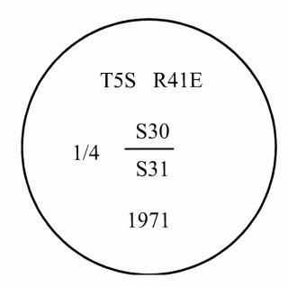
I used a steel tape and magnetic compass in the establishment of the bearing trees. Magnetic declination used was 13° East. Bearing is to a brass washer marked OPLS 83571 in the lower blaze of the tree. Distance is to a spike set in the root crown of the side of the tree.
