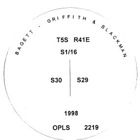
I used a steel tape and compass with 17° E magnetic declination in the establishment of the new accessories. The distances are to a 60d spike driven into the right side of the root crown of the bearing tree. I attached a brass washer marked OPLS 2219 to the BT blaze.
