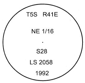
I used a steel tape and magnetic compass in the establishment of the new accessories. I used  $14^\circ$  East declination, the distances are to a 60d spike driven into the right side of the root crown of the bearing trees. A brass washer marked OPLS 83571 is attached to the BT blaze of the new bearing trees.
