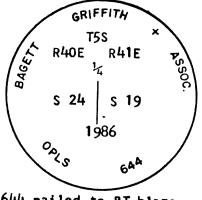
Brass washer marked OPLS 644 nailed to BT blaze. Used steel tape and magnetic compass with 200 East declination. Distances to the BTs are to a 50d spike set in right side of tree when facing tree, unless otherwise stated.
