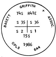
Brass washer marked OPLS 644 nailed to BT blaze. Used steel tape and magnetic compass with 20° East declination. Distances to the BTs are to a 50d spike set in right side of tree when facing tree, unless otherwise stated.
