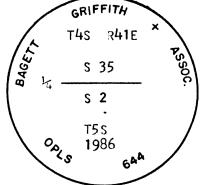
Brass washer marked OPLS 644 nailed to BT blaze. Used steel tape and magnetic compass with 20° East declination. Distances to the BTs are to a 50d spike set in right side of tree when facing tree, unless otherwise stated.
