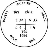
Brass washer marked OPLS 644 nailed to BT blaze. Used steel tape and magnetic compass with  $20^{\rm O}$  East declination. Distances to the BTs are to a 50d spike set in right side of tree when facing tree, unless otherwise stated.
