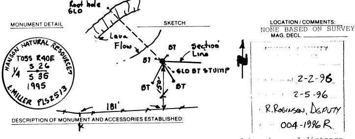
At the original corner point determined at record bearing and distance from the original bearing trees as described above. I set a 3"0.D. x 12" galvanized iron pipe, 6" in the ground to solid rock, with a 3" brass alloy cap, stamped as shown on the DETAIL. The pipe is surrounded by rock above and below the ground surface and secured in place with cement.
