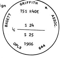
Brass washer marked OPLS 644 nailed to BT blaze. Used steel tape and magnetic compass with 20° East declination. Distances to the BTs are to a 50d spike set in right side of tree when facing tree, unless otherwise noted.
