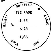
Brass washer marked OPLS 644 nailed to BT blaze. Used steel tape and magnetic compass with 20° East declination. Distances to the BTs are to a 50d spike set in right side of tree when facing tree, unless otherwise noted.
