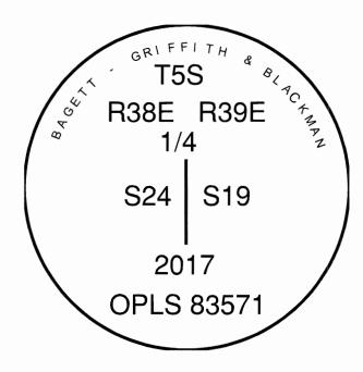
I used a steel tape and magnetic compass in the establishment of the bearing trees. Magnetic declination used was 13° East. Bearings and distances are to the center of the tree.
