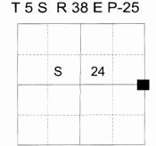
location. I buried the pipe to within 8" above the surface of the ground. I then placed a mound of stone 3 1/2 feet dia. and 1 foot high covering the monument. From which I set two new bearing trees:
