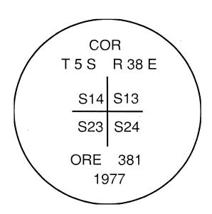
I used a steel tape and magnetic compass in the establishment of the new accessory. I used 16° East declination, the distances are to a 60d spike driven into the right side of the root crown of the new bearing trees. A brass washer marked OPLS 83571 is attached to the BT blaze of the new bearing trees.
