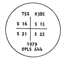
Brass washer was nailed to B.T.blaze. Used steel tape and magnetic compass with 18 East declination.
