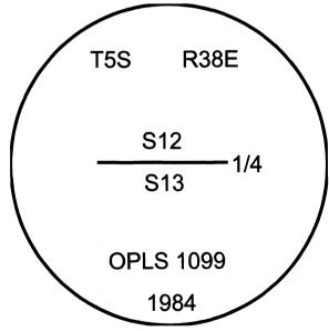
I used a steel tape and magnetic compass in the establishment of the new accessories. I used 14° East declination. Distances are to a 60d spike driven into the right side of the root crown of the bearing trees. Bearings are to a brass washer marked OPLS 83571 in the BT blaze of the new bearing trees.
