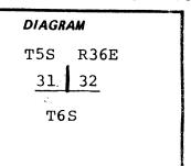
Description of corner evidence found: Cap is stamped: 3" brass Cap on 2 3/8" iron pipe rising 10" above ground. No stones available. Steel fence post 2 ft. east of corner. COR T6S R36E T5S BT's found: S31 S32 a dead & down pine, badly decayed, bears N71°W, S6 8 lks., blaze, scribing faintly visible.
