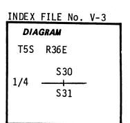
Description of corner evidence found: Found 15"x12"x4" stone with faint "1/4" mark on North face. Stone has fallen onto its west side. Restored stone to upright position and located 24" Pine stump with foot blaze but no scribing bearing  $S81^{OW}$ , 12.8 ft. Also old Pine stump 16" in dia. bearing  $N53^{OE}$ , 25.2 ft. with foot blaze mark and no scribing.
