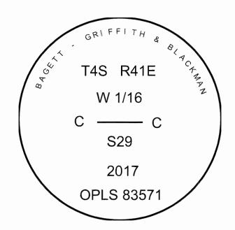
I used a steel tape and magnetic compass in the establishment of the bearing trees. Magnetic declination used was 13° East. Bearings are to a brass washer marked OPLS 83571 in the lower blaze of the new trees. Distance is to a spike set in the root crown of the side of the new trees.
