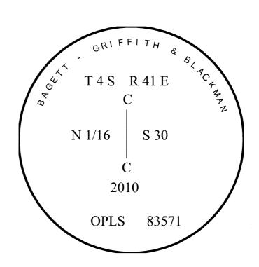
I used a steel tape and magnetic compass in the establishment of the accessories. I used 16° East declination, the distances are to a 60d spike driven into the root crown at the right side of the bearing trees. I place a brass washer marked OPLS 83571 in the lower BT blaze.
