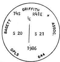
Brass washer marked OPLS 644 nailed to BT Blaze. Used steel tape and magnetic compass with 20° Ea declination. Distances to the BTs are to a 50d Spikeset in right side of tree when facing tree, unless otherwise stated.
