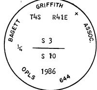
Brass washer marked OPLS 644 nailed to BT blaze. Used steel tape and magnetic compass with 20° East declination. Distances to the BTs are to a 50d spike set in right side of tree when facing tree, unless otherwise stated.
