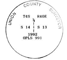
I used a steel tape and magnetic compass in the establishment of new accessories. I used 17° East magnetic declination and the distances are to a 50d spike driven in the right side of the root crown. I attached a brass washer marked OPLS 991 to the BT blaze.
