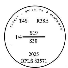
I use a tape and compass in the establishment of the new bearing objects. 14° East was used for declination and measured to a brass washer labeled "OPLS 83571" in the BT blaze at the base of the tree. Distances are to a 60D nail in the right wide of the base of the center of the tree.
